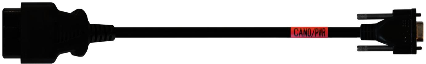
The Influx OBDII Type B to 9 way D Type Cable can be used to connect power and the Diagnostics CAN bus of a vehicle to the Rebel Dash or a K-Box. It can also be used to connect to the CAN0/PWR port of a Multi Connect Cable to connect power and the Diagnostics CAN bus of a vehicle to a current Rebel CT or LT Logger. Type B connectors may be plugged into both 12V and 24V Vehicles.
