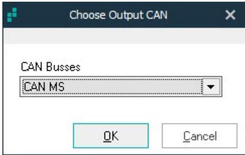
CAN Buses—Drop down menu selects the Output CAN Bus from the available connections on the Rebel Data Logger.
