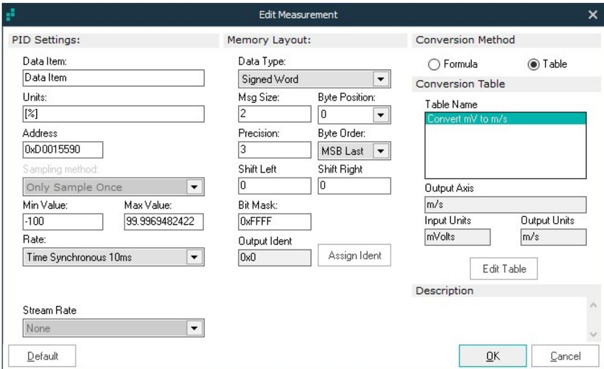
The screenshot shows the 'Edit Measurement' dialog box with the 'Conversion Method' tab selected. The 'Table' radio button is chosen. The 'Conversion Table' list contains one entry: 'Convert mV to m/s'. The 'Output Axis' is set to 'm/s', 'Input Units' to 'mVolts', and 'Output Units' to 'm/s'. There is an 'Edit Table' button below the list. The 'Description' field is empty. At the bottom right are 'OK' and 'Cancel' buttons.
